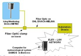
Fig. 4: Communication between ice monitoring device and main computer
