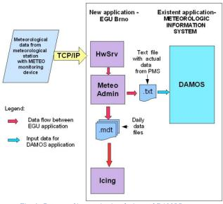
Fig. 4: Concept of ice monitoring device and DAMOS system
